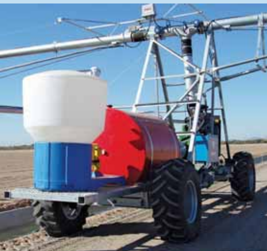
Rainger ditch feed with auxiliary platform and chemigation
