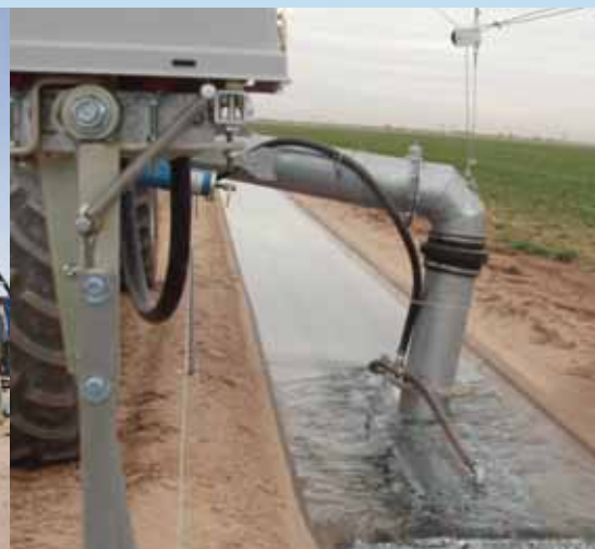
Rainger ditch feed with above ground guidance and rolling suction
