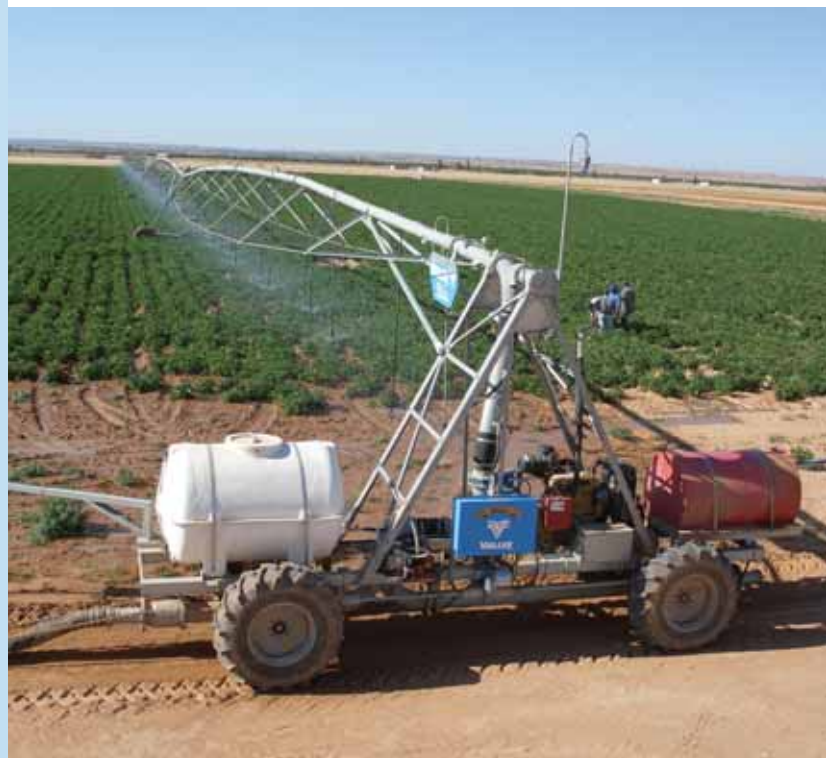
Rainger hose drag with cart mounted booster pump
