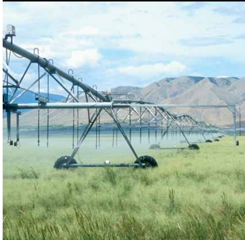
Linear span with below ground guidance
