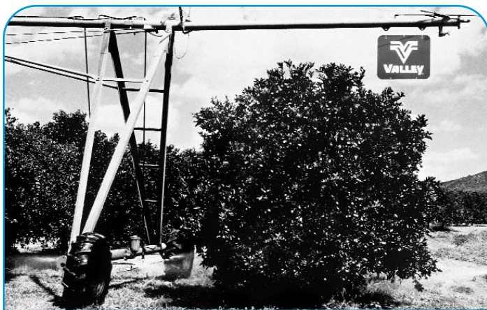
High profile center pivots can irrigate trees as high as 5 meters tall.
