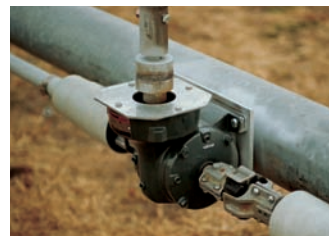
Center drive powered by the spinner mechanism.
